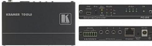
The FC-26 is a PoE-powered control gateway, capable of plug and play deployment over a customer Ethernet LAN for remote control of customer controlled devices via bidirectional RS-232 and IR control connections. Multiple control clients can be IP-connected to the FC-26 control gateway for concurrent control of two RS-232 and four IR controllable devices, such as AV scalars, video displays, audio amplifiers, and DVD players
